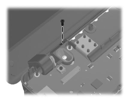
Where used: 1 screw that secures the speaker assembly to the base enclosure
